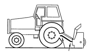
Equal Angles at Driveline Joints
