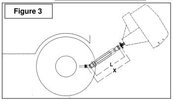
**NOTE:** Before cutting, make sure the two shafts intersect by at least 7 3/4" when in working position that is when the snowblower rests on the ground.
