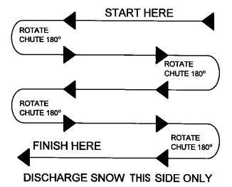
If the snow can only be thrown to one side of the driveway or sidewalk (above), start on the opposite side. At the end of the first pass, rotate the discharge guide 180 degrees for the return pass. At the end of each succeeding pass, rotate the discharge guide 180 degrees to maintain direction of throw in the same area.
