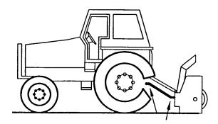
Equal Angles at Driveline Joints <u>Recommended</u>
