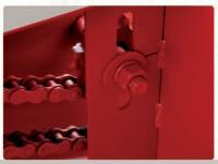
**Drive chain** | Blizzard snowblowers have an easily accessible manual chain idler on the side of the snowblower housing for quick adjustment.
