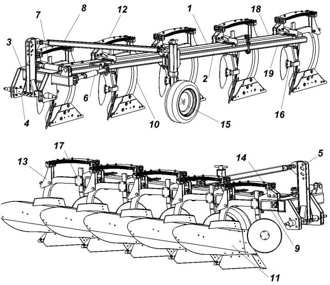
Figure 1. 1-beam plough - general construction: 1 - main frame, 2 - subframe, 3 - coupler head, 4 - suspension axle, 5 - three-point suspension system rack, 6 - longitudinal adjustment screw (or hydraulic actuator), 7 - transversal adjustment screw, 8 - stay, 9 - body handle, 10 - leg, 11 - body, 12 - suspension spring, 13 - spring rear handle, 14 - spring front handle, 15 - support wheel, 16 - rolling skimmer, 17 - skimmer handle, 18 - body main frame +1, 19 - body subframe +1
