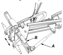
Figure 7. Ploughing width adjustment; A - actuator, B - turnbuckle
