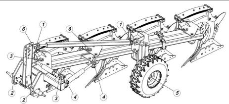
Fig. 9. Lubrication points
