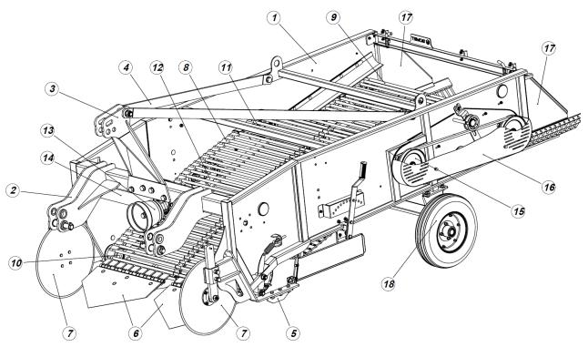
Figure 1. 2-row conveyor digger: 1 - frame, 2 - three-point suspension system lower brackets, 3 - three-point suspension system rack, 4 - stay, 5 - ploughshare holder, 6 - ploughshare, 7 - disc coulters, 8 - front sieving conveyor, 9 - rear sieving conveyor, 10 - tension roller, 11 - drive roller, 12 - shakers, 13 - angle gear, 14 - intermediate shaft, 15 - belt transmission, 16 - transmission metal shield, 17 - chute grate, 18 - axle with road wheels
