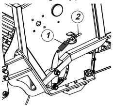
Fig. 2. Adjusting the conveyor tension
