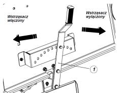
Fig. 4. Adjusting the sifting intensity
