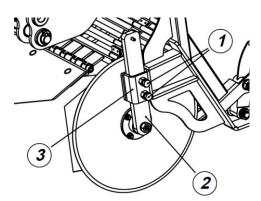
Fig. 3. Adjustment of disc coulter
