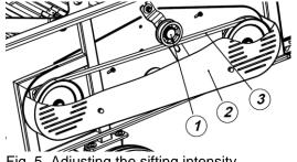
Fig. 5. Adjusting the sifting intensity
