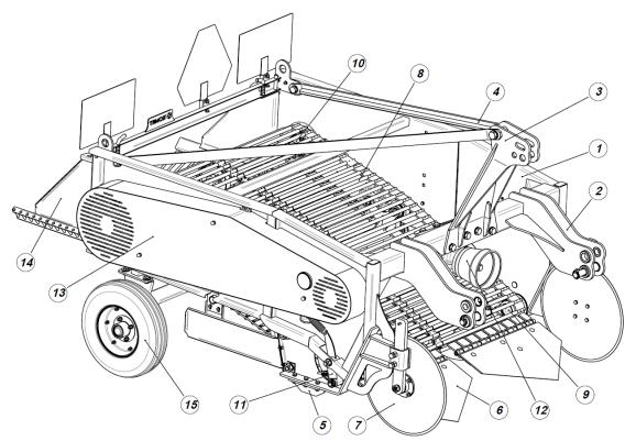
Figure 2. 2-row conveyor digger with 1 conveyor: 1 - frame, 2 - three-point suspension system lower brackets, 3 - three-point suspension system rack, 4 - stay, 5 - plowshare holder, 6 - plowshare, 7 - disc coulters, 8 - front sieving conveyor, 9 - tension roller, 10 - drive roller, 11 - shakers, 12 - angle gear, 13 - belt transmission with shield, 14 - chute grate, 15 - axle with road wheels
