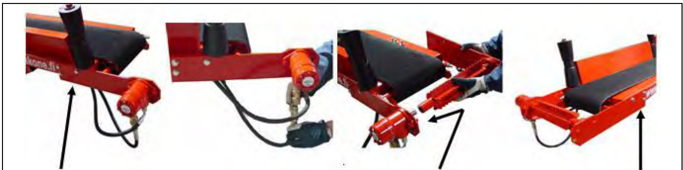
Figure 4. Installing the auxiliary input roller
