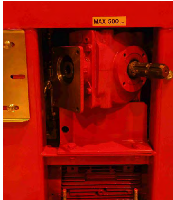
Figure 23. Replacing the angle transmission
