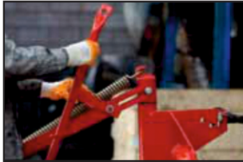
Figure 7- Disconnect the tension spring (1)
