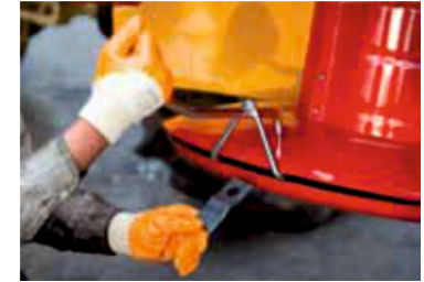
Figure 17- Replacing the knives
