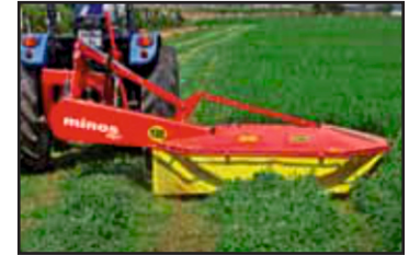
Figure 9- Lowering of the Mower from the transport into the working position, (3)
