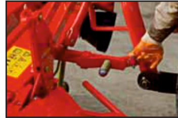
Figure 8- Connect the tension pin and control (2)
