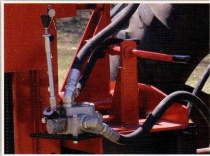
Offset controls allow the operator to stand safely to the side of the unit while posts are being driven.
