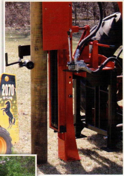
The driver is mounted on a base plate that allows the unit to tilt in two directions, making it easy to drive posts straight—even in uneven terrain.
