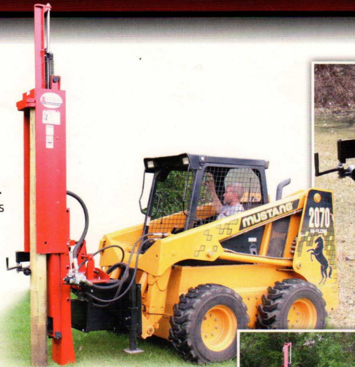
New stabilizer leg offers greater stability and decreases driving time.
