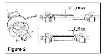
Always couple the two end yokes of the driveline and check that they are locked in place.
