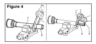
4. If driveline must be cut to a shorter length, clamp driveline in a well padded vise to prevent damage to the shield. Cut off shield where marked. Using cut-off section of shield as a guide, cut shaft the same amount. (Figure 4.)
