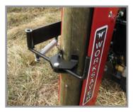
Post Holder - Spring loaded arm holds post securely for "hand free" operation.
