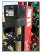
Rubber Shield — First to install rubber shield around ram driving head, reduces flying wood chips and debris.
