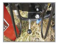
Bubble Level - First with a circular bubble level on all units for simple, yet accurate positioning of the driving ram.
