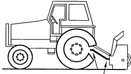
**Equal Angles at Driveline Joints**
