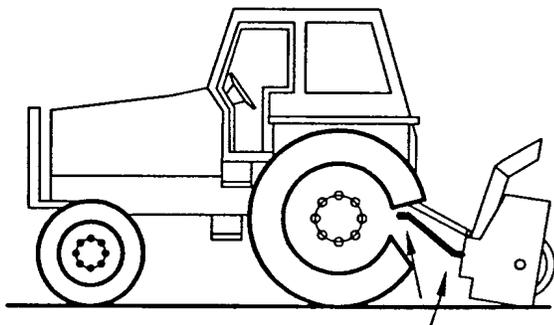
**Unequal Angles at Driveline Joints**
