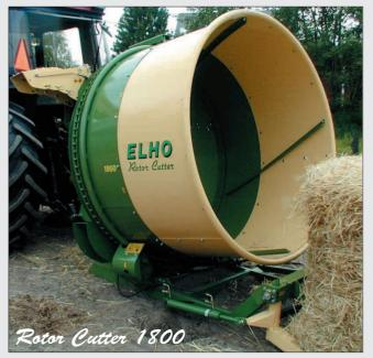
The heavy sprocket drive between the hydraulic motor and the drum, together with the solid guide rollers ensure the even rotation of the drum, and so also the even distribution of the chopped bales. The rotation speed of
