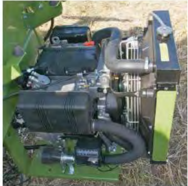
The ELHO Tube 2020 is available either with an 11 hp petrol engine or 16 hp Lombardi Diesel engine. They both have electric start as standard.
