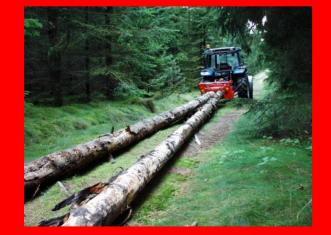
The grapple will easily handle logs up to 20-30 mtr / 60/90 ft. The swing cylinder of the grapple must be connected to a float section of the tractor's hydraulic valve assembly.
