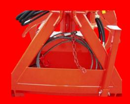
HZ-2300 and HG Models have a transport box build ind the 3-point hitch. For cable slings and forestry chains etc.
