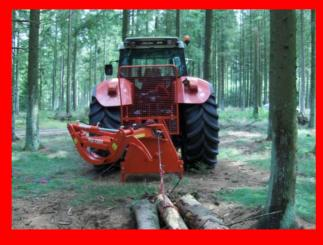
All VHZ and VHG models includes a 3-ton forestry winch on the 3-point hitch, which is operated by displacing the claw to the left and is activated manually by pulling the green power cord.
