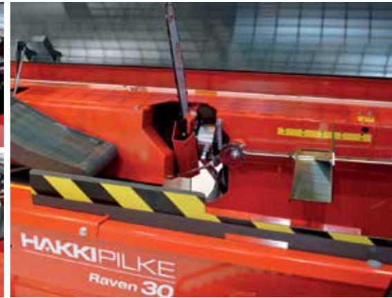
The log press holds the wood firmly in place when cutting thin logs. Space is provided around the drive end to enable easy blade maintenance.
