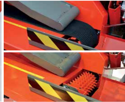
Log feed with a belt on Standard and Deluxe models (above), and with a spiked roller in the Basic model (below).
