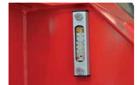
Large oil tank capacity and sight glass.
