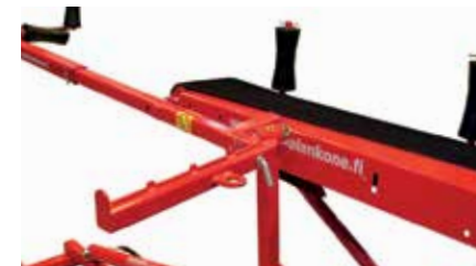
The support is integrated inside the arm.
