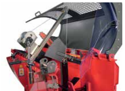
Replacing the splitting blade is fast and safe thanks to the detachable winch.
