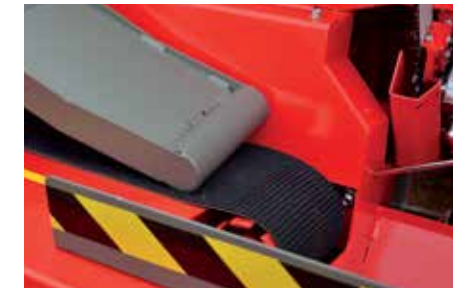
Log feed using a heavy duty belt with a rough surface.
