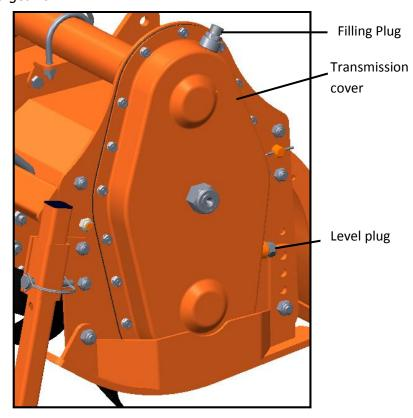
Check the oil level every 50 hours, making sure it reach's the level plug on the transmission cover.
