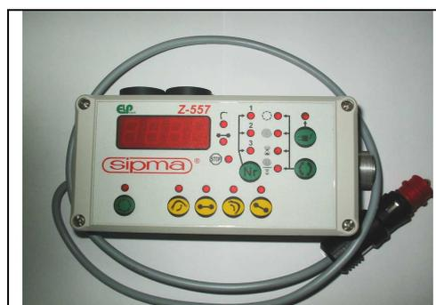
Fig. 36 Wrapping machine controller
