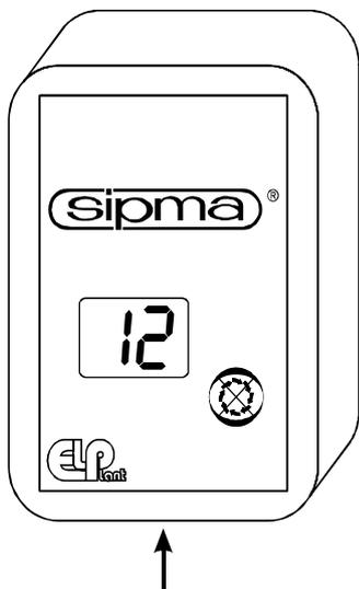
To turn the device on plug the sensor cable into the socket on the bottom of the casing.
