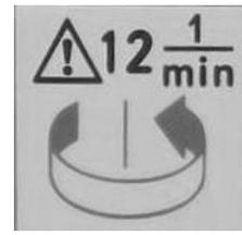
Fig. 11 Direction and number of revolutions.
