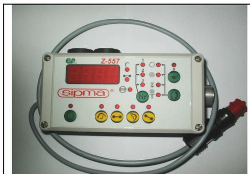
Fig. 36 Wrapping machine controller
