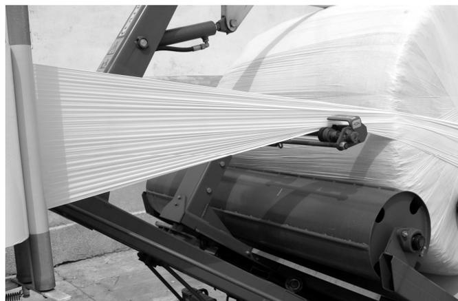
**Fig. 34 Positioning of the foil in catcher - clipper by tipping the frame**
