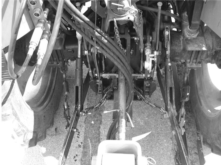
*Fig. 26 Coupling the bale wrapping machine with the tractor*
