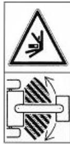
**Fig. 6. Stand clear from the area of the joint hitches**
