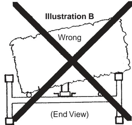
**SOLUTION:** Load bales as shown in Illustration A above or use a Bale Chute accessory (*Model No. HST-5A or HST-12A*), as shown below.
