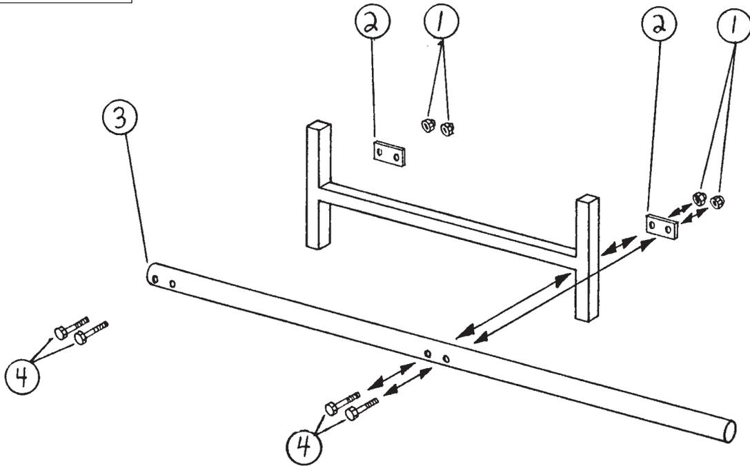
It is important that the motor mount pipe be installed as shown below so as to assure proper fitting of shield.
