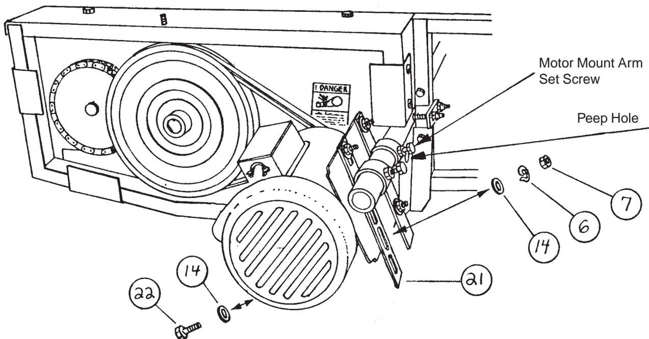
Look through peep hole (under motor mount pipe) in lower shield, and determine the belt is in line. Also check that belt is snugged up but not overtightened. OVERTIGHTENED BELTS WILL CAUSE BEARING AND PULLEY FAILURE.
