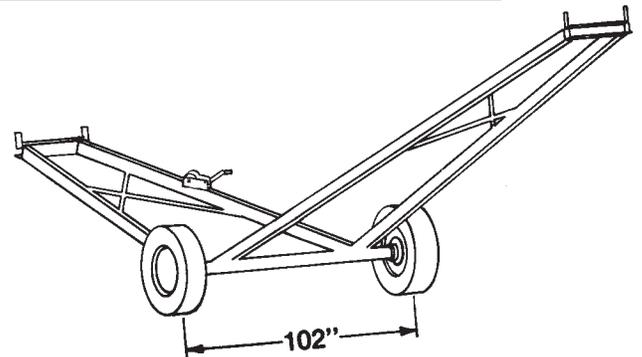
*(From center of tire to center of tire - outside width will vary depending on tire width)*
