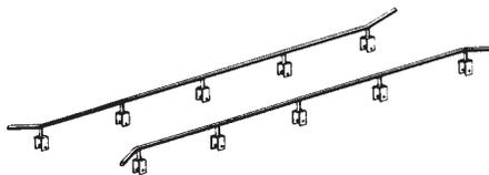
**Bale rails:** Rails increase height of elevator sides to prevent irregular-shaped bales from tumbling out. Rigid 12" long steel rails clamp onto sides of inclined elevator.
