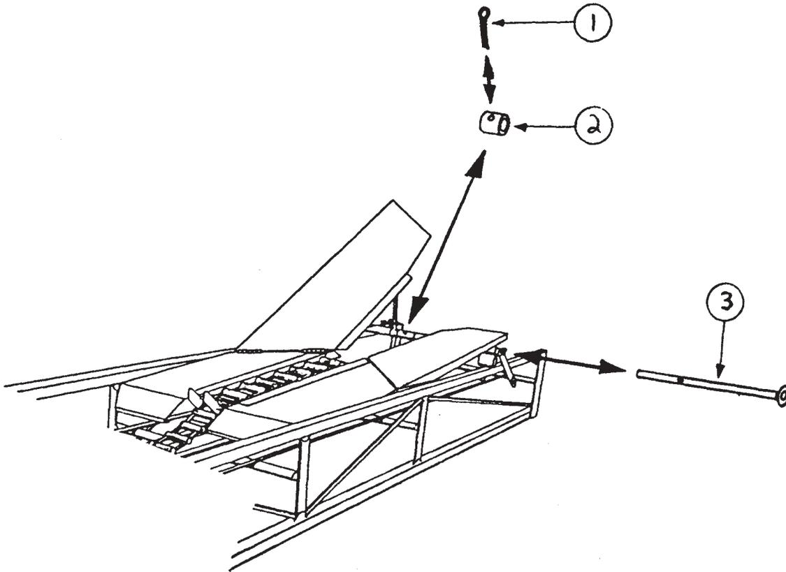
Tapered design provides for unloading to either right or left along conveyor. Kick-off may be removed from or installed onto conveyor without breaking the conveyor chain. Remove cotter pin #1 and pull out kick-off axle #3 and spacer #2. Lift conveyor chain up from conveyor chain track. Conveyor chain should ride over green plastic wear strip and under kick-off axle. Reassemble kick-off axle, spacer and cotter pin.
