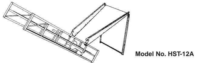
**Bale chute (grate-type, 6' length):** Hinges to elevator — tips back against wagon or truck for easy unloading. Long-taper design automatically lines up each bale to prevent them from tipping or turning while being conveyed up elevator. Grate-type construction permits loose material to fall through for smoother operation.
