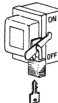
**Lockout:** A main power disconnect switch capable of being locked only in the OFF position shall be provided. This shall be locked whenever work is being done on the equipment.
