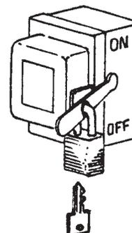
**Lockout:** A main power disconnect switch capable of being locked only in the OFF position shall be provided. This shall be locked whenever work is being done on the equipment.
