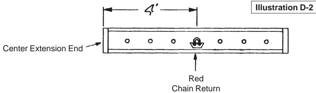
Bolt one red chain return #49 onto underside of each 4' center extension, 2' from center extension end (refer to Illustration D-3 below).
