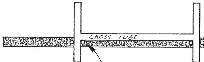
Check and make sure that the 5/16" x 3" bolts are pressed tight against the bottom side of cross tube.
