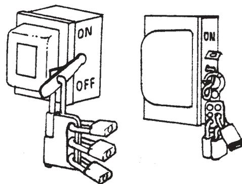
Attaches to main power disconnect switch. Equipment cannot be started until all workmen have removed their personal padlocks.
