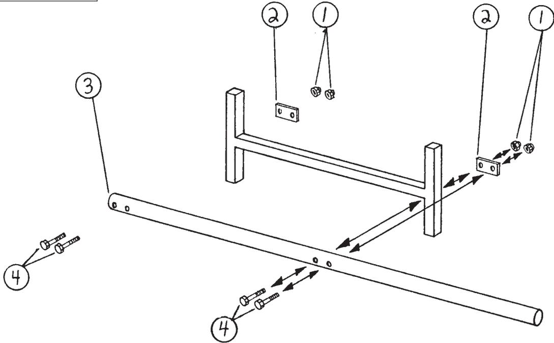
It is important that the motor mount pipe be installed as shown below so as to assure proper fitting of shield.
