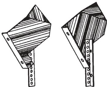
**Connector plates:** Connects incline elevator to horizontal mow conveyor. Prevents bales from turning and tumbling out when transferring.
