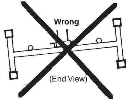
**SOLUTION:** Clamp conveyor to a solid wood mow-hanger as shown below. Locate wood mow-hanger near motor drive end of conveyor, as weight imbalance (due to motor) is greatest at that point. Wood mow-hangers are not available from the factory.
