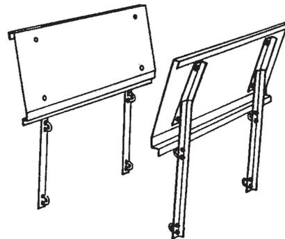
**Bale arrangers:** Directs irregular shaped bales into horizontal conveyor. Made of heavy galvanized steel.
