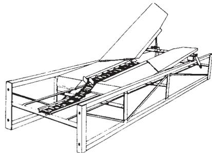
**Bale kickoff** Sturdy, tapered design provides for fast, smooth, accurate unloading to either right or left from any point along conveyor. Pull control rope (rope not included), from mow floor to change direction of unloading or to slide kickoff to any position along full length of conveyor. Bales cannot be conveyed over kickoff and onward toward end of conveyor.
