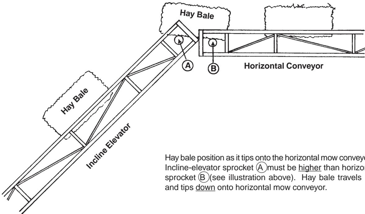
Hay bale position as it tips onto the horizontal mow conveyor is very important. Incline-elevator sprocket (A) must be higher than horizontal mow conveyor sprocket (B) (see illustration above). Hay bale travels up incline-elevator and tips down onto horizontal mow conveyor.
