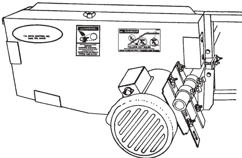
Elevator should be securely fastened to the building during operation or when raised and unattended. This machine is not insulated. Keep away from overhead electrical wires and devices. Electrocutation can occur without direct contact. If shields are lost or missing, contact T. R. Metal Crafters, Inc. for free replacement.
