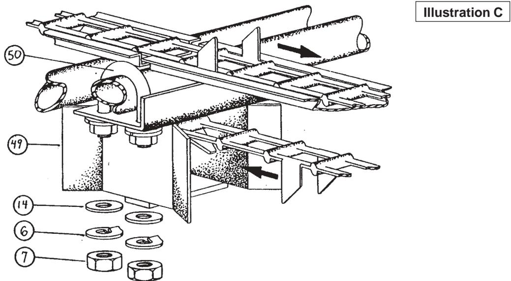
Bolt one red chain return #49, onto underside of 8' drive section, 6' from drive sprocket end (refer to Illustration D below).
