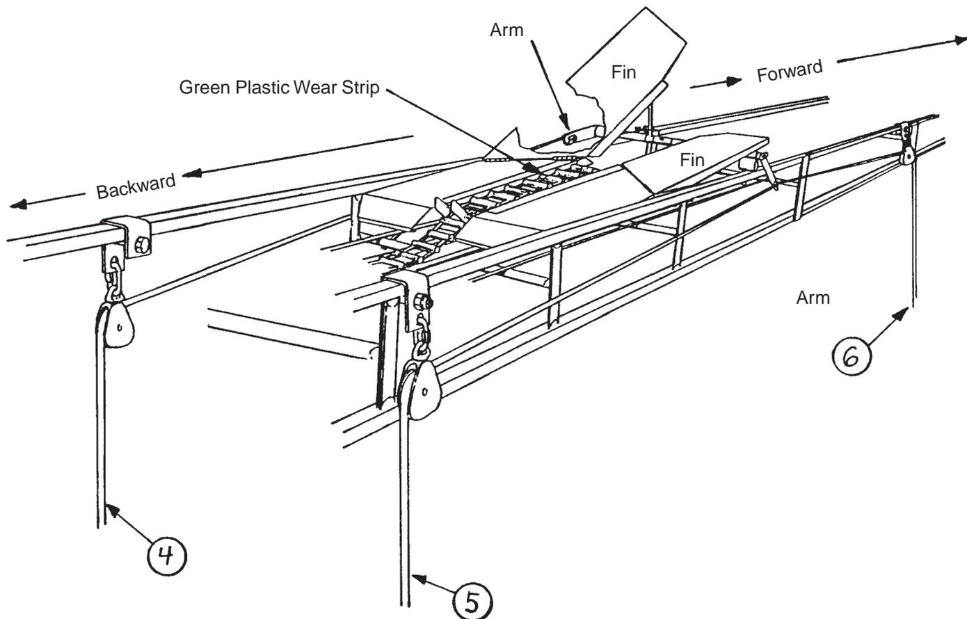
Each kick-off requires 3 control ropes. Use a 1/4" low-stretch grade, nylon rope. The length of each control rope is equal to the conveyor length plus distance of conveyor to barn floor. Install control ropes as shown in the following illustrations.
