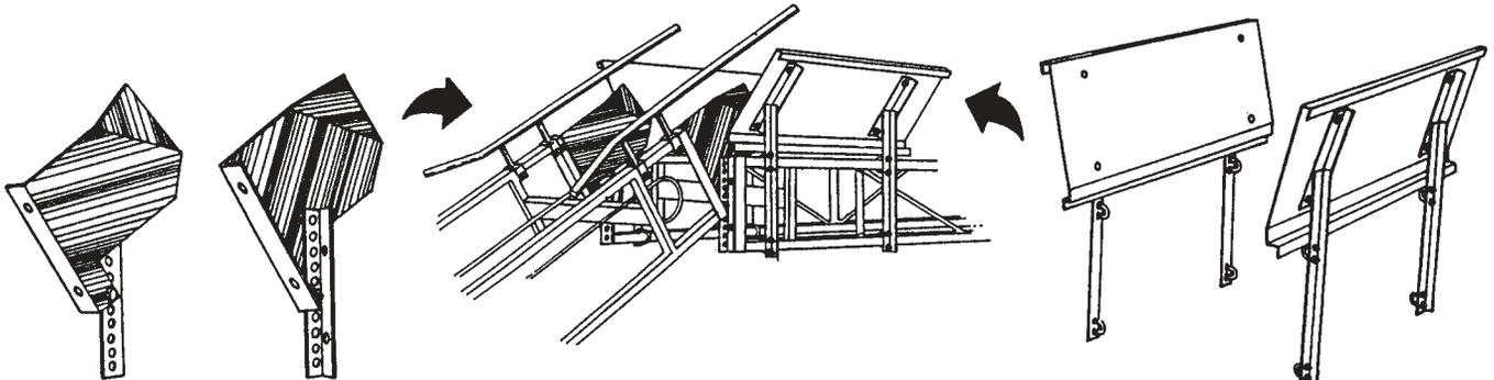
**Connector plates:** Connects incline elevator to horizontal mow conveyor. Prevents bales from turning and tumbling out when transferring.
