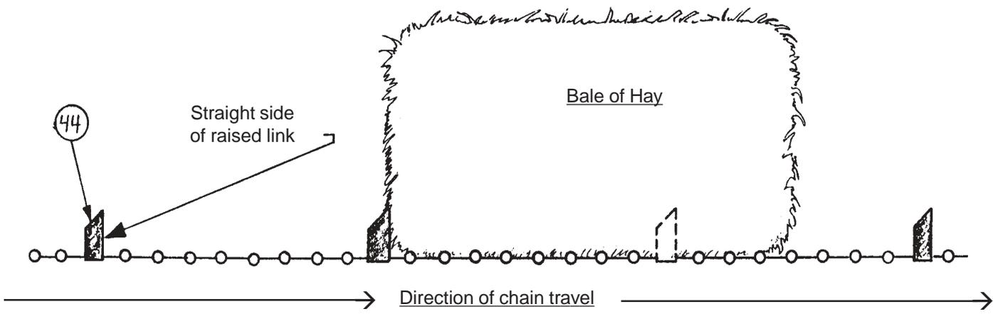
The chain can then be assembled and fished through the red chain returns on bottom of elevator. Connect and tighten chain until snug.
