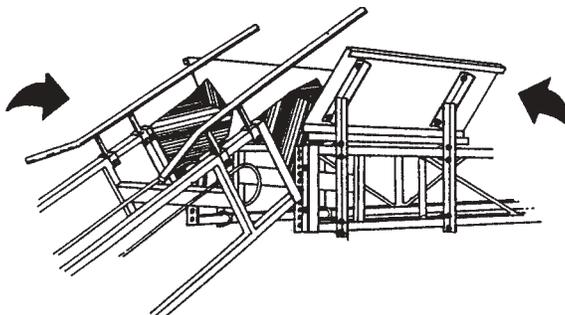
Above drawing illustrates incline elevator assembled to horizontal conveyor, using Bale Guides (model HST-7A), Connector Plates (model HST-17A or 18A) and Bale Arrangers (model HST-16A).
