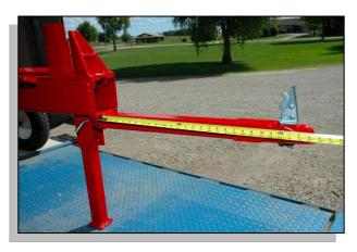
Extended Nose Hitch Tongue extensions are available upon request. This is useful for towing behind All Terrain Vehicles (ATV) or lawn tractors. Hitch options include Pintle Hitch and 1 7/8" couplers. Also available is an 800lb swivel jack with a 6" wheel which helps in handling larger and heavier model wood splitters.
