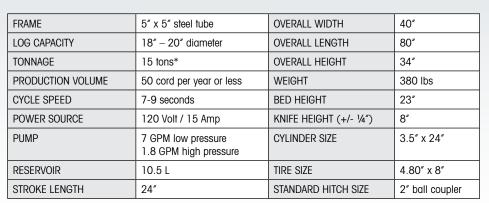
\* Rated tonnage comparable to 15 ton rated standard log splitters. Options include log lifter, heavy duty suspension, 4"or 8" raised bed height, 24" nose extension, swivel jack, pintle hitch
