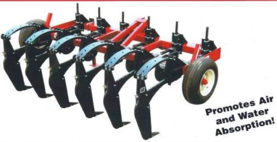
TEBBEN'S New Zone Till Shank fractures compacted ground while leaving residue on top. Tebben Enterprises Automatic Reset Shank Assembly will trip over rocks and other obstacles while maintaining up to a 22" digging depth. Front cutting coulters ahead of each shank helps leave surface residue and soil relatively undisturbed.
