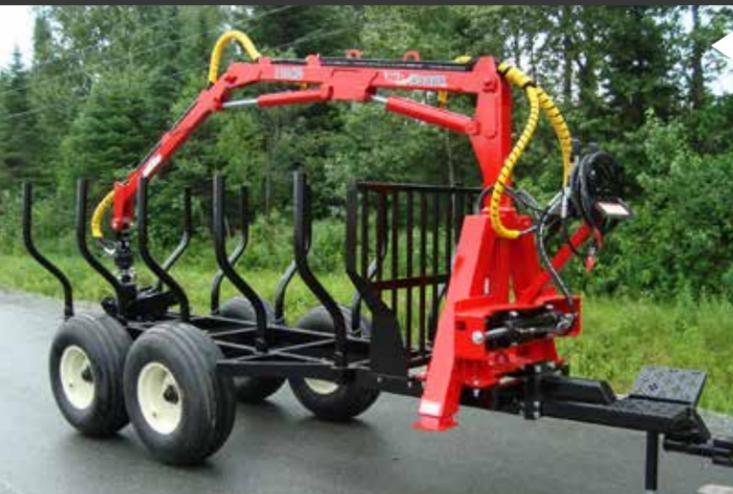
The 115-HD Woody Log Loader is part of the Intermediate series. Primarily designed for tractors from 30 hp to 70 hp, but can easily adapt to 50 hp to 70 hp tractors if work sites are in areas such as mountainsides with steep slopes. Lightweight, but also as well equipped as the larger industrial models, the 115-HD Log Loader is an excellent compromise between the Compact series and the Industrial series.
