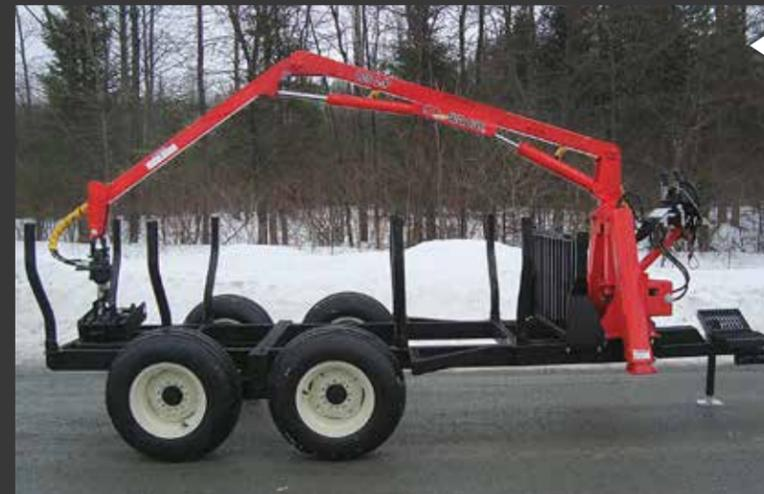
The 125-LP Low Profile Woody Log Loader was specifically designed with maple producers in mind. Its low profile boom and lowered trailer allow it to easily pass under the tubes making it very convenient when working in the sugar bush.
