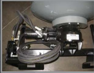
Worksaver's Skid Steer Mixer, model SS-590 has direct hydraulic drive of the gearbox which eliminates chain and sprocket maintenance resulting in more up-time on the jobsite. Large 11-cubic ft. drum allows the operator to mix, transport and place 5-cubic ft. of concrete. It's efficient design offers the contractor a cost savings over chain driven models.
