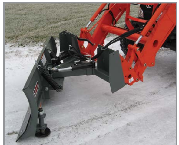
Adjustable skid shoes are standard
