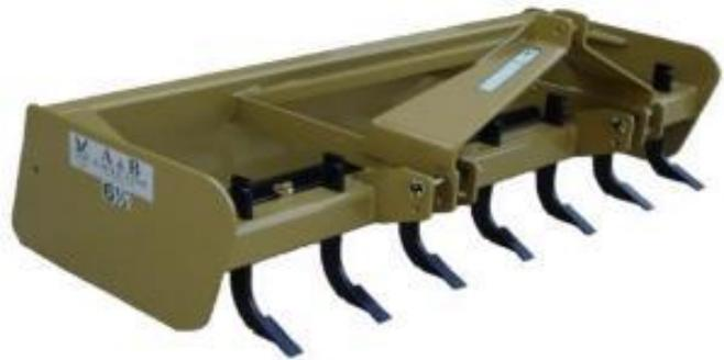
**\* ALL WELDED, NO ASSEMBLY REQUIRED \* CAT. 1/ 2 COMBINATION HITCH \* FLOATING OR LOCKED REAR MOLDBOARD \* SCARIFIER SHANKS ARE ON 11" CENTERS \* FRONT MOLDBOARD ROLL FORMED FOR ADDED STRENGTH AND IMPROVED SOIL FLOW \* REAR MOLDBOARD IS DOUBLE FORMED FOR ADDED STRENGTH \* SCARIFIER SHANKS ARE QUENCHED AND TEMPERED WITH 3 DEPTH SETTINGS**
