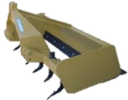
**\* ALL WELDED, NO ASSEMBLY REQUIRED \* CAT. 1 / 2 COMBINATION HITCH \* SCARIFIER SHANKS ARE ON 11" CENTERS \* FRONT MOLDBOARD ROLL FORMED FOR ADDED STRENGTH AND IMPROVED SOIL FLOW \* REAR MOLDBOARD IS DOUBLE FORMED FOR ADDED STRENGTH \* SCARIFIER SHANKS ARE QUENCHED AND TEMPERED WITH 3 DEPTH SETTINGS**
