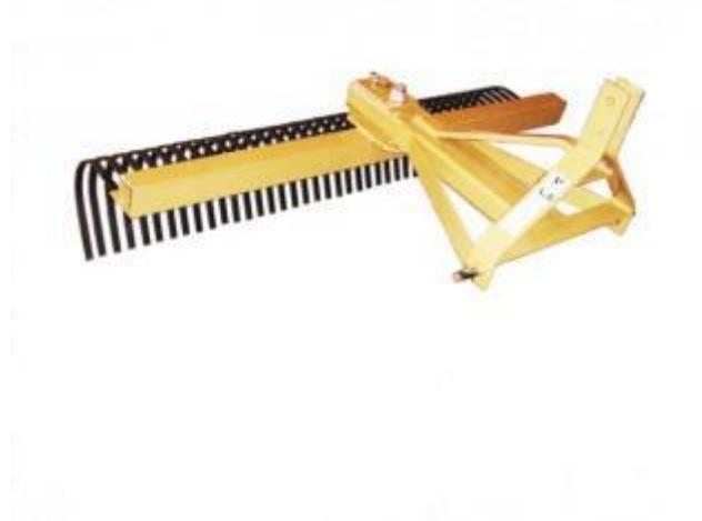
**\* COMES ASSEMBLED, ADD A-FRAME AND READY TO USE \* QUICK HITCH READY \* TEETH ARE HEAT TREATED SPRING STEEL \* LOCKING CLAMP TO PREVENT SIDE MOVEMENT OF RAKE TEETH \* ALL BOLTS HAVE STEEL LOCK NUTS TO REDUCE LOOSENING FROM VIBRATION \* 3 POINT HITCH A-FRAME AND REPLACEABLE LIFT ARM PINS**
