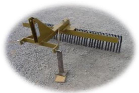
\* COMES ASSEMBLED, ADD A-FRAME AND READY TO USE \* QUICK HITCH READY \* TEETH ARE HEAT TREATED SPRING STEEL \* LOCKING CLAMP TO PREVENT SIDE MOVEMENT OF RAKE TEETH \* ALL BOLTS HAVE STEEL LOCK NUTS TO REDUCE LOOSENING FROM VIBRATION \* COMPACT 3 POINT HITCH A-FRAME AND REPLACEABLE CAT. 1 LIFT ARM PINS \* STAND NOT INCLUDED
