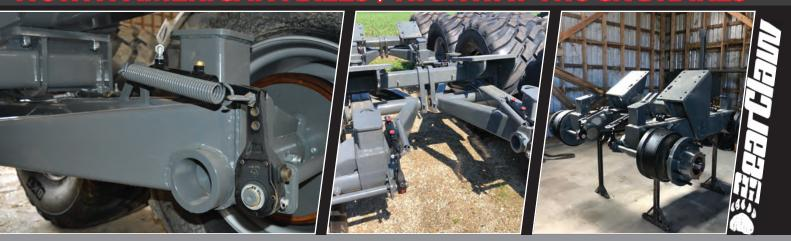
North American axles / Highway truck brakes: Makes spare wheels and axle/brake parts easier to find. Removable stub axles for any major repairs.
