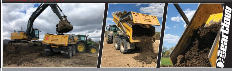
Tapered body, helps to reduce the drag on the walls when dumping, the load ejects easier and at a lower height than straight walls.
