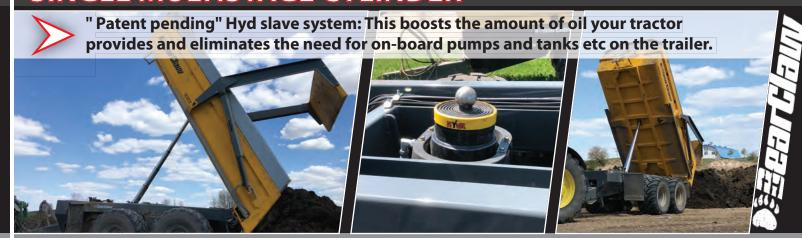
Single, Multi-stage dump cylinder: Requires less oil from the tractor, accommodating older, smaller tractors with limited oil capacity.
