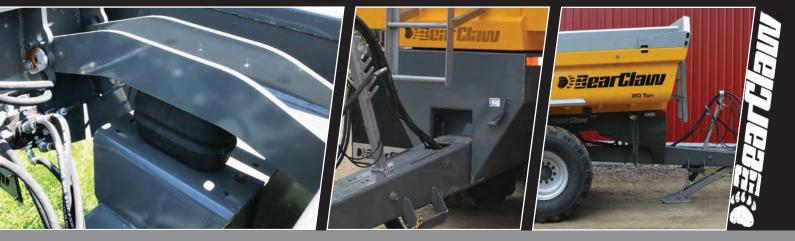
Adjustable rubber ride hitch: Reduces jumping on the hitch through rough ground or at speed.
