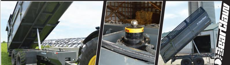
Single, Multi-stage dump cylinder: Requires less oil from the tractor, accommodating older, smaller tractors with limited oil capacity.
