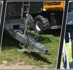
Adjustable rubber ride hitch: Reduces jumping on the hitch through rough ground or at speed.
