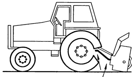
**Equal Angles at Driveline Joints**
