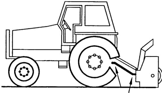
**Unequal Angles at Driveline Joints**
