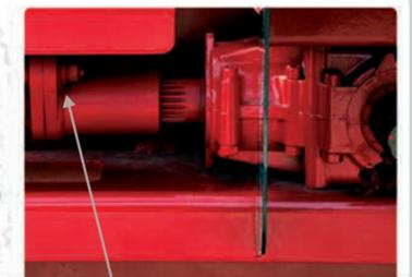
**Shear bolt** protection on the drive shaft to prevent costly repairs.
