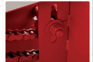
**Drive chain** | Blizzard snowblowers have an easily accessible manual chain idler on the side of the snowblower housing for quick adjustment.
