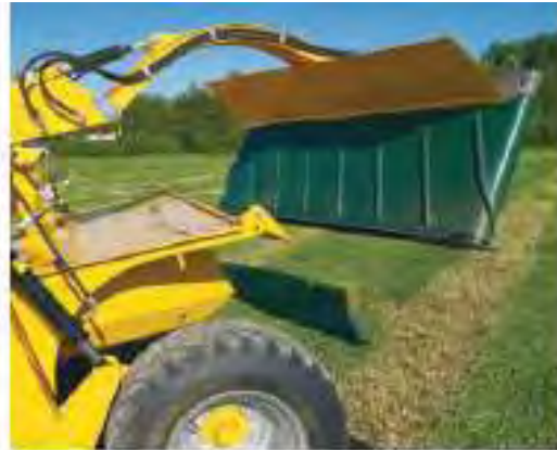
The ELHO Arrow 3700 is an effective trailed mower conditioner, added with ELHO's SideFlow III cross conveyor the harvesting can be made even more effective. The SideFlow III can also be reversed, and it has its own hydraulics and oil tank.
