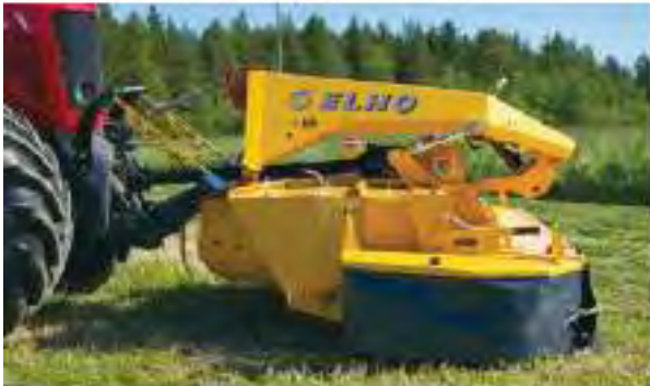
ELHO's Arrow Front mower conditioners have the PCS three-point suspension, so that the sides can move freely and the machine can avoid obstacles easier. The HydroBalance system is the standard equipment of the machine.
