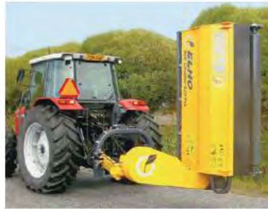
Transport position with double locking.
