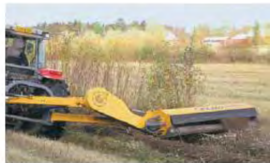
Even the thicker small trees present no problem to SideChopper. There are two knife alternatives. The 1.3 kg high-quality hammer knives come as standard. YI knives are optional accessories that are suitable for grass fallow land and thicket cutting.
