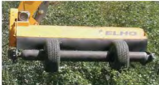
The wear runners made of 16 mm Hardox guarantee a long service life.
