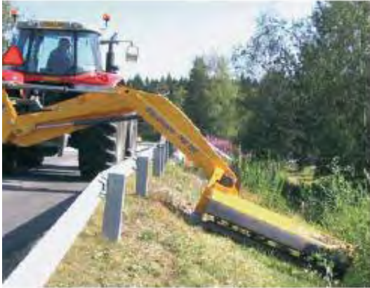
SideChopper TPM520 Pro reaches over fences of different heights, often even to the slope on the opposite side.
