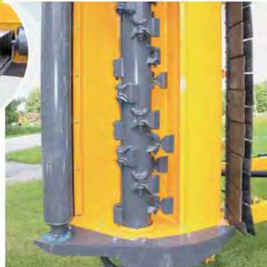
Even the thicker small trees present no problem to SideChopper. There are two knife alternatives. The 1.3 kg high-quality hammer knives come as standard. YI knives are optional accessories that are suitable for grass fallow land and thicket cutting.
