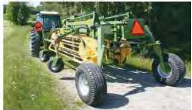
Force steered rear wheels, low centre of gravity, as well as low and narrow structure make the V-Twin 750 extremely easy to drive on the road. Changing from the transport position to the working position and vice versa is very fast. There is no need to come out of the cabin during the position change.
