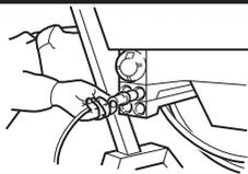
**Make sure that the hydraulic pipes are fitted and mounted correctly. If they are inverted this will cause movements opposite to those commanded.**
