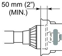
If the PTO shaft supplied with the machine is not being used, check that the cowlings of the machine and of the tractor are overlapped on the protection of the PTO shaft at least by the amount contemplated by the safety regulations in force (50 mm/1.97 in).
