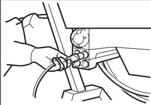
Ensure that the hydraulic pipes are correctly fitted, respecting the colour recognition code and remembering that inverting them causes opposite movements to those ordered with the controls.
