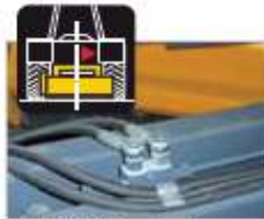
Hydraulic block valve for transport with automatic activation (no chains or holders).
