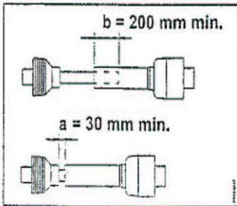
The P.T.O must be cut to a proper length, so it does not "bottom out" and bind. Remove the PTO to perform this operation. If the PTO is not cut to the proper length, it may cause damage to the PTO, gearboxes etc. See illustration for proper measurements.
