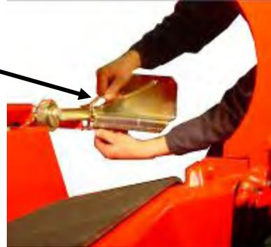
**NOTE! When the wood diameter exceeds 30 cm, turn the limiter!**
