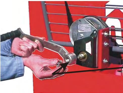
Install the crank for the conveyor winch (no. 8 in Figure 2) by screwing it into place, and lock it with a nut. **Note! Do not fully tighten the nut. Leave a 3 mm clearance between the crank and the nut!**
