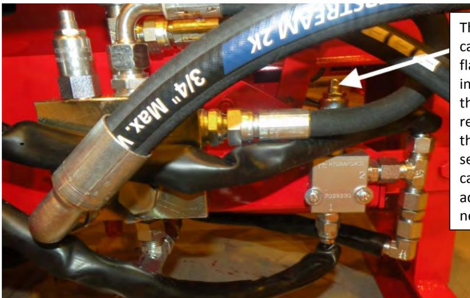
The pressure adjustment cartridge for the cutting flange's downward motion. To increase the pressure, tighten the hex socket screw. To reduce the pressure, loosen the screw. There is no separate design value for the cartridge. The operator should adjust the pressure as necessary.
