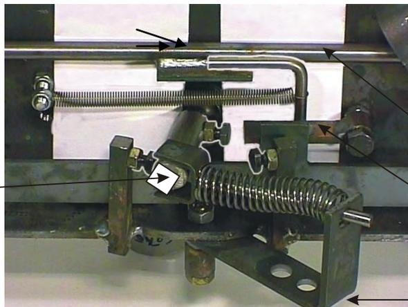
5. When the jointed lever is on the left, the trigger lever and trigger rod are lowered to the initial position.
