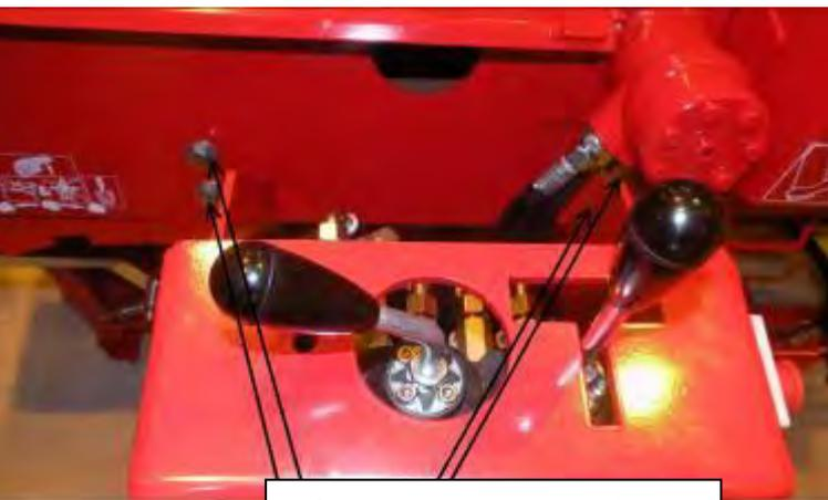
Lift the control panel into place, and fasten it with four bolts.
