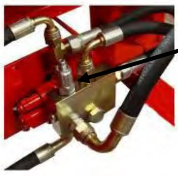
3. Open the locking nut of the acceleration valve's adjustment bolt.
