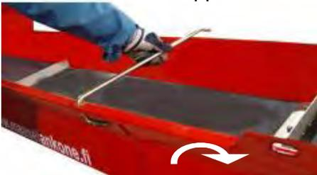
CHECK THE CONDITION OF THE CONVEYOR WINCH AND ITS COMPONENTS ON A DAILY BASIS. IF YOU DISCOVER A FAULT, NO MATTER HOW SMALL, REPLACE THEM.
