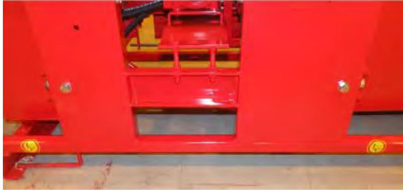
*Figure 3. Lifting points for a forklift.*
