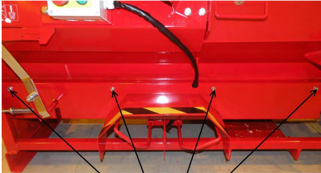
Install the pedal guard (no. 5 in Figure 1) with four bolts as shown in the figure.
