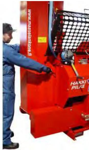
2. Push the conveyor towards the splitter, and release the conveyor lock by lifting the locking handle.
