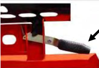
3. Lift the input conveyor guard, and ensure that the guard is locked in the raised position.
