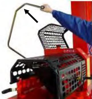
The input conveyor is activated when the cutting lever is moved up from its initial position. Note! In the Easy model, the conveyor can be activated with the control lever B (in Figure 20) by pushing the lever to the up/right position.
