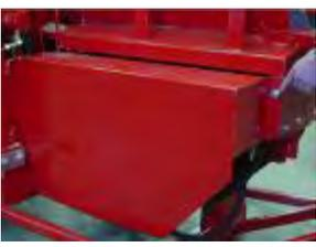
1. Remove the locking bolt of the valve unit's cover.
