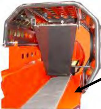
The wood press keeps the logs in place when they are being sawed. Do not put your hand between the wood press roller and the input conveyor belt!
