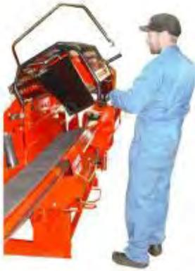
Ensure that the feed conveyor guard is properly locked in the raised position!
