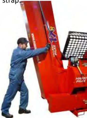
3. Pull the conveyor until the winch strap tightens.
