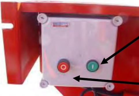
The splitter will not start with the green switch unless the stop switch at the front of the machine is disengaged.
