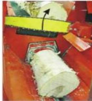
Automatic - set off as the splitting blade starts to rise from its lowest position.
