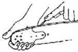
Clean the flange groove and the lubricating oil channel
