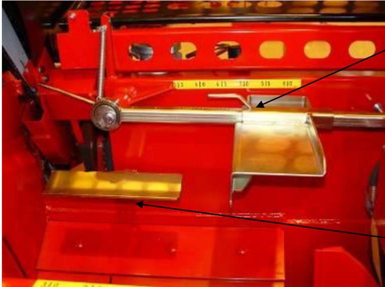
Locking bolt. Remove the bolt pin from below to lift the bolt.
