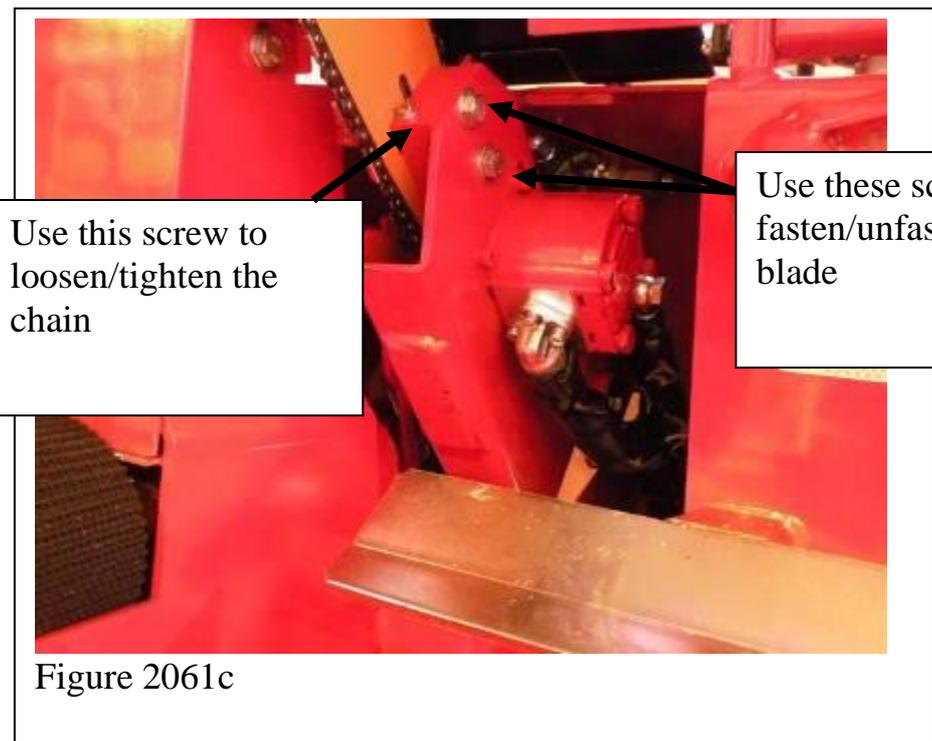
Use this screw to loosen/tighten the chain
