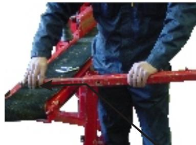
2. Remove the cotter and pin from the beam which is closest to the operator.
