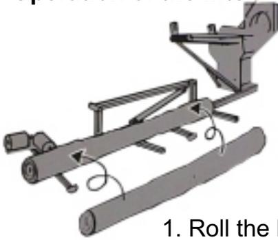
1. Roll the log onto the lifter.
