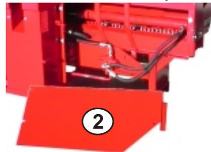
2. Remove the cover of the hydraulic system.
