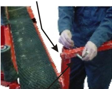
2. Remove the cotter and pin from the beam which is closest to the operator.
