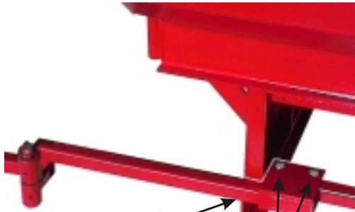
1. Fit the lug for attaching the lifter to the frame of the machine.
