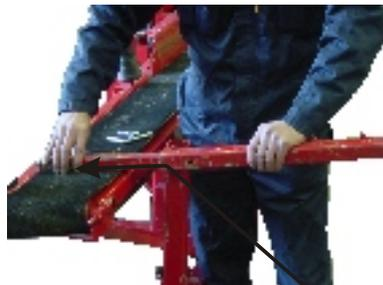
3. Pull out the beam extension onto the top of the infeed conveyor, align the hole in the lifting beam with the hole in the extension and put the pin through both these holes.
