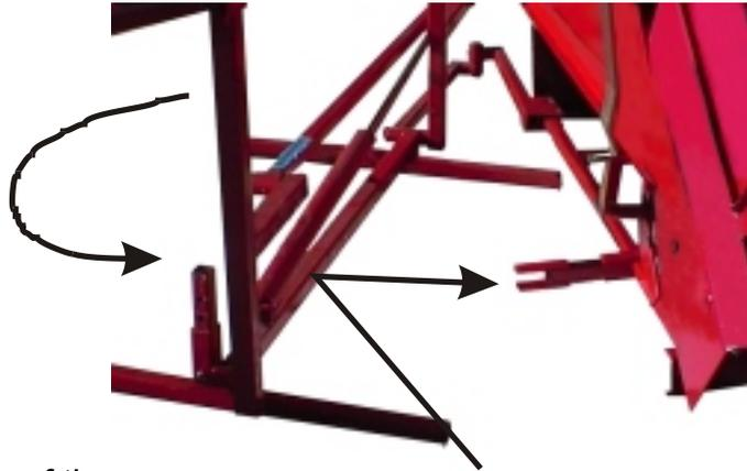
3. Place the pipe on the lower frame of the lifter in the lug on the lower frame of the machine.
