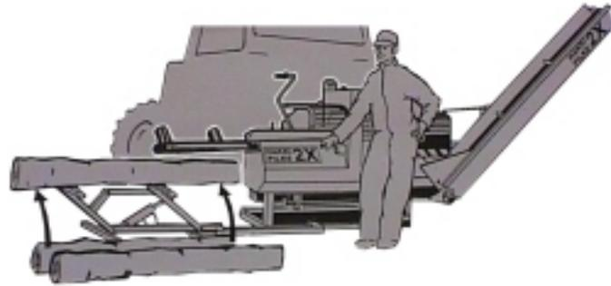
2. Raise the log onto the machine using the lifter. During lifting, always make sure that the rising log can neither hit you nor damage the machine.
