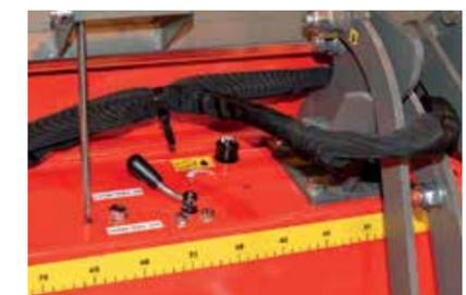
The AC 10 automatic chain tensioner maintains optimal saw chain tension at all times. The chain can be conveniently replaced with the lever shown in the picture – no tools required!
