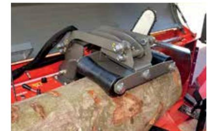
The hydraulic log press enables logs of all sizes to be sawed effortlessly.
