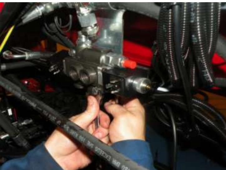
8. Remove the attachment bolts of split valve (2 pcs).
