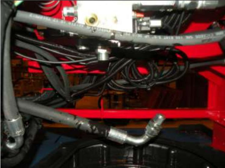
4. Remove the hydraulic hoses of speed valve and mount the plug (3/4") for the hose, which goes to hydraulic oil tank. Like in figure above.
