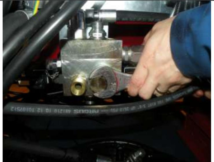
5. Remove the attachment bolts of speed valve and remove the speed valve from the split valve.
