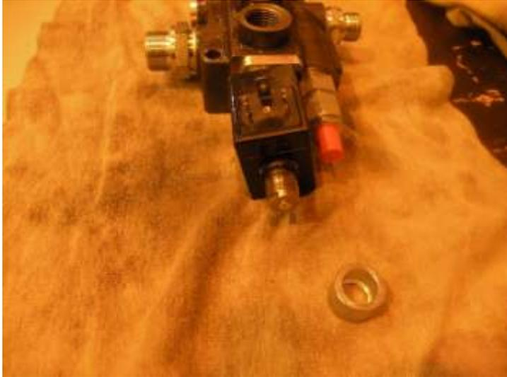
10. Remove the attachment nut of inductor and pull inductor and O-ring off (from both side of shaft).
