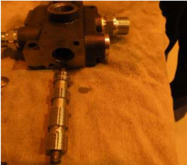
12. Pull the shaft off. You can also test that the shaft isn't too tight to move.
