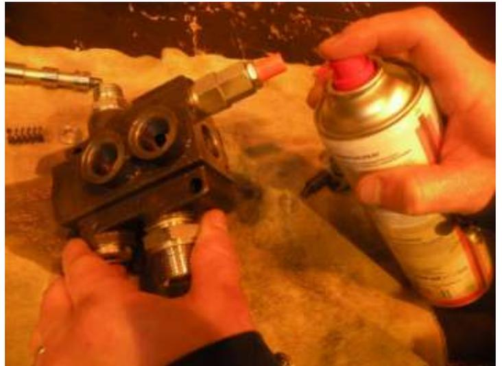
13. Spray a cleanser (e.g. Brake Spray) into valve from every opening and blow also pressure air at the end. Then mount the pieces in reverse order.
