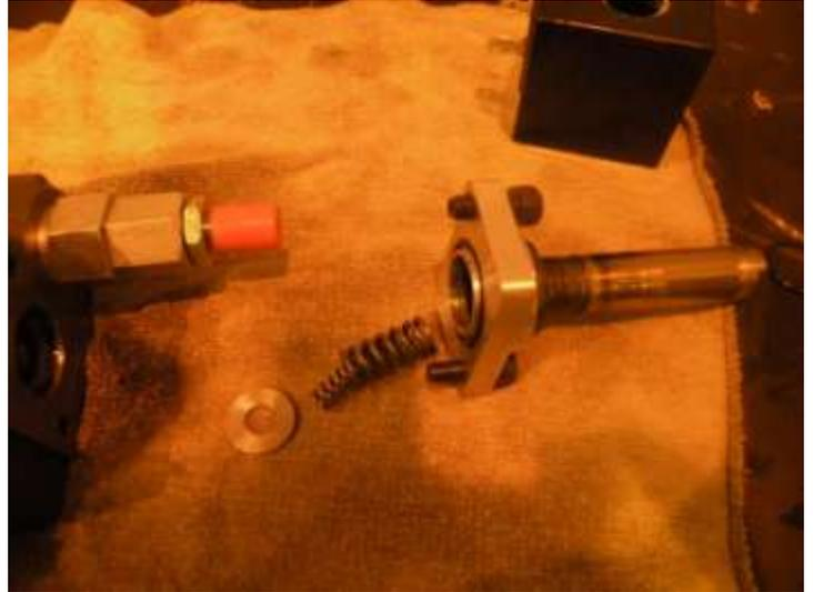
11. Remove the shaft of inductor, springs and washer. (N.B there's only 1 spring on the other side).
