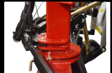
**DOUBLE SHEAR ANGLE CYLINDER MOUNT**
