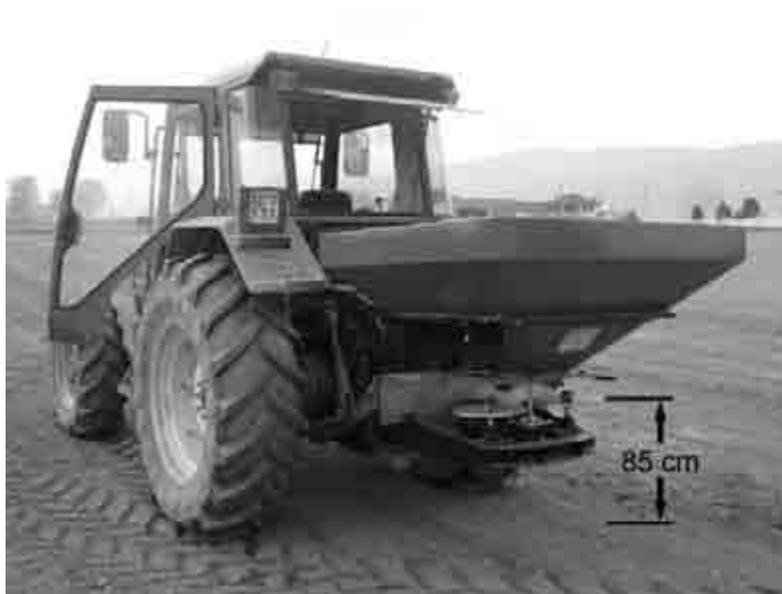
**85 cm between the ground level and the distribution disk height**
