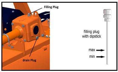
If the sign is below the minimum, fill up oil till restore the correct level.
