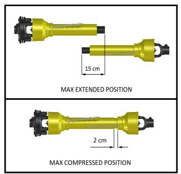
A driveshaft too long may cause structural damages to the tractor and machine. If the driveshaft is too long, it may be adapted by removing it and shortening the tubes according to the instructions provided by the manufacturer in its use and maintenance manual.
