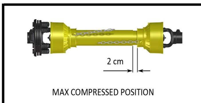
A driveshaft too long may cause structural damages to the tractor and machine. If the driveshaft is too long, it may be adapted by removing it and shortening the tubes according to the instructions provided by the manufacturer in its use and maintenance manual.
