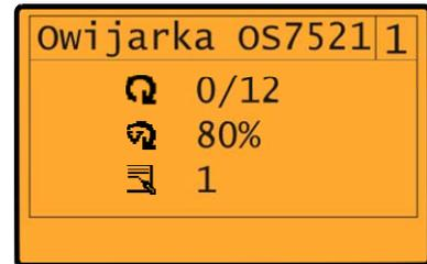
The parameter of relative rotational speed of the table is on the first automatic mode screen entitled " Wrapping machine OS-7521" in the second line of parameters from the top. This parameter can be edited only when the terminal displays automatic mode windows. Editing is performed with the use of two yellow keys on the left side of the display (without description).
