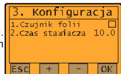
If the film sensor is selected as active ( - square with a dot) when during wrapping impulses from the sensor generated by rotating film roll cease to appear, the table will stop and the screen will show a screen informing about film rupture.
